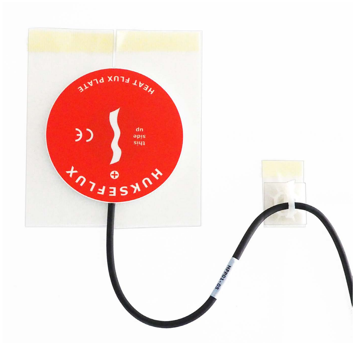
Figure 5.1.1 Installation of HFP01 on a wall using sided “removable” carpet laying tape such as TESA 4939, and a strain relief of the cable using a cable tie mount equipped with the same carpet laying tape as adhesive.
