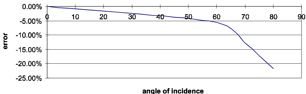
FIGURE 4. Cosine Response of a Typical Net Radiometer
