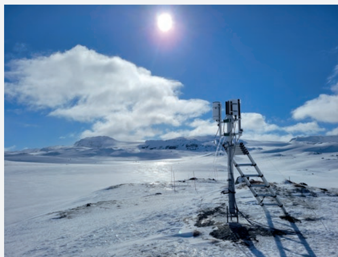
Figure: Solar UV+visible+near-infrared monitoring at Finse Research Station. Hardangerjøkulen in the background.
