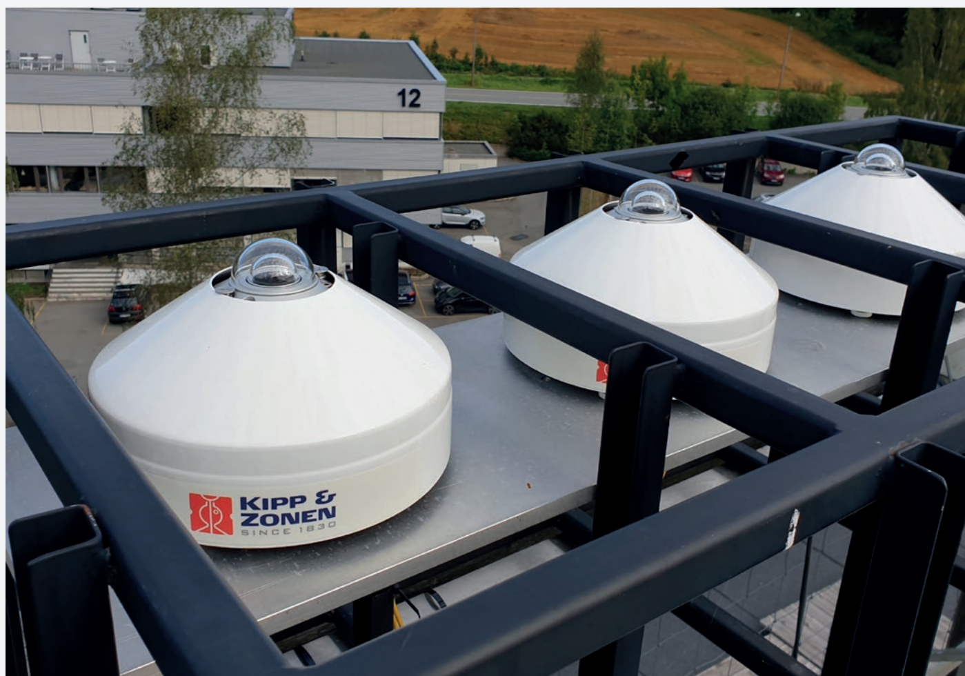
Figure: Testing pyranometers (total solar radiation) before installation at UV-network stations.
