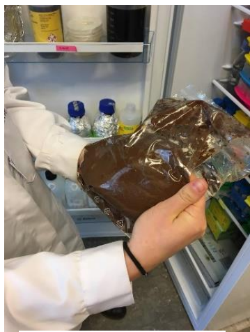
Raw material for enzymatic degradation of cellulose and hemicellulose from Norwegian Spruce Photo: Christine K. Kristiansen
