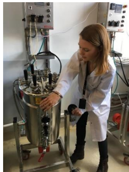
Newly recruited Bio4Fuels PhD student Line D. Hansen next to a 30 liter reactor used for high-dry matter enzymatic saccharification reactions. The biorefinery at NMBU allows experiments at small pilot scale and is part of the national NorBioLab infrastructure for biorefining.
