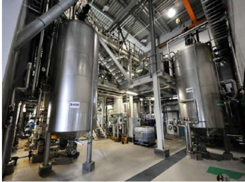
Borregaard's Demo Unit in Sarpsborg, which was used to showcase faster and more complete saccharification of Borregaard's BALI-pretreated spruce feedstock at demonstration scale, using the recently developed industrial setup, enabling controlled activation of LPMOs in Novozymes' CellicCTec3 cocktail using H 2 O 2 supply. Photo by Martin Lersch, Borregaard.
