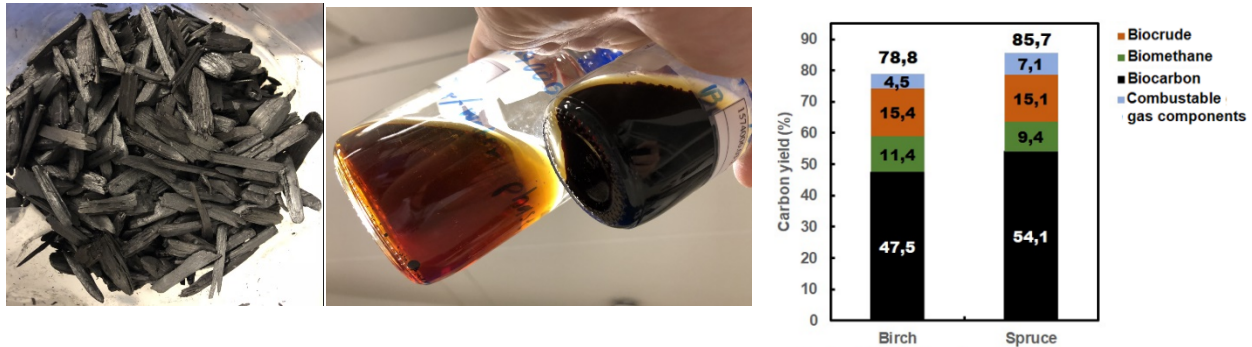
a) Photo: The Bio4Fuel research team at RISE PFI are exploring coproduction of biogas transportation fuel, biocrude and biocarbon by combining intermediate pyrolysis technology and anaerobic digestion a) Biocarbon and condensate intermediate pyrolysis byproducts b) Carbon product yields obtained in coproduction of biogas transportation fuel, biocrude and biocarbon from Norway Spruce and Birch wood.
