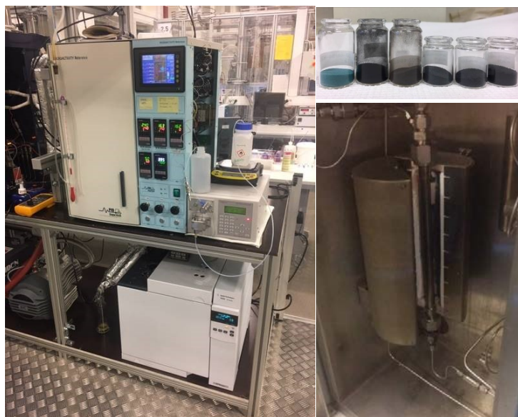
Photo: Catalyst testing setup (left) , copper based catalyst materials (upper right) and the fixed bed reactor (lower right) for testing catalysts activity.
