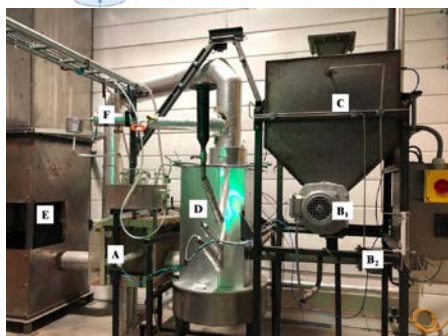
Figure 2: Fluidized bed gasification reactor at USN Porsgrunn
