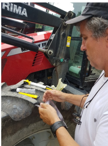
Checking tractor-motor wear during the biodiesel test by analyzing the oil quality (photo: Bondelaget).
